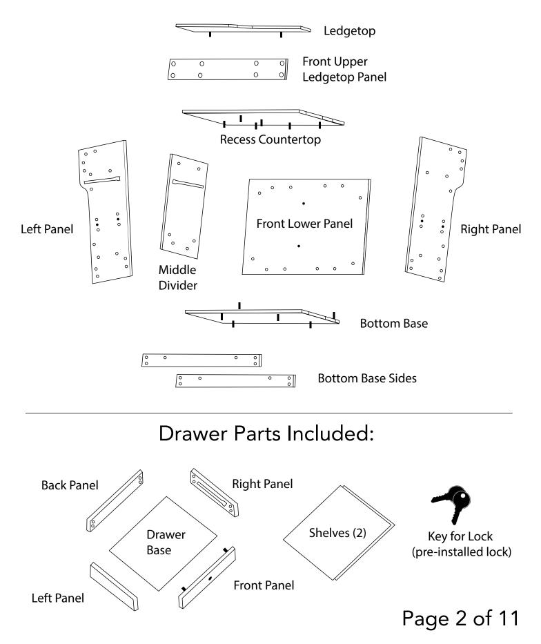
Screw cam lock pins in small holes of bottom base. Set bottom base sides on top of bottom base camlock pins. Make sure arrows on cam lock nuts are facing to the right. Then tighten with screw driver. Note: Hardware on bottom base sides should point inward. (See Diagrams)
