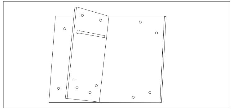
Line up front lower panel and middle divider on top of the bottom base camlock pins. Make sure arrows on cam lock nuts are facing to the right. Then tighten with screw driver. (See Diagram 3A)
