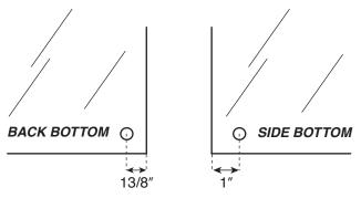
MEASURE THE GLASS SPACE BETWEENEDGE OF GLASS AND CENTER OF HOLE. HOLE FURTHEST FROM EDGE GOES ON BOTTOM.
