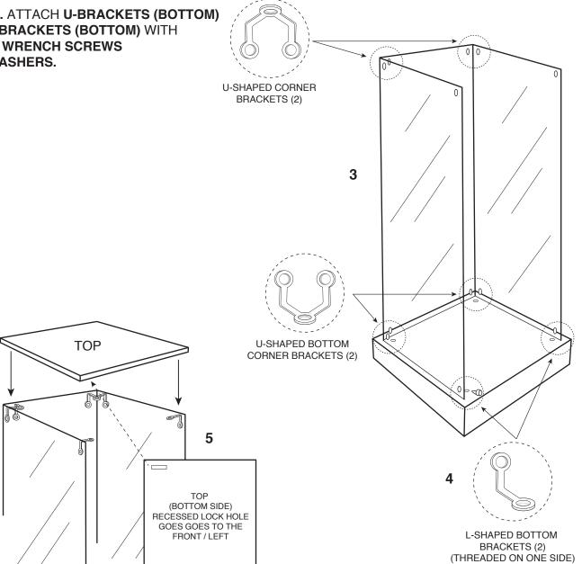
STEP 5. PLACE TOP ONTO ASSEMBLY. ATTATCH WITH ALLEN SCREW AND PLASTIC WASHERS AND L-BRACKETS.
