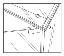
ATTACH **TOP RIGHT** OF FRONT DOOR (APPROXIMATELY 1/16" FROM EDGE OF GLASS) - **REPEAT** HINGE ASSEMBLY ON BOTTOM
