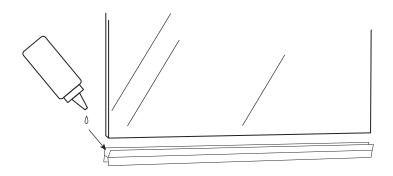
RUN BEAD OF ANY TYPE OF GLUE ON INSIDE (BOTTOM) OF TOP PLASTIC SLEEVE. THEN TAP SLEEVES ON TOP OF THE GLASS WITH A RUBBER MALLET.
