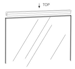
PLACE METAL SLEEVES (WITH LOCK TO THE LEFT) ON BOTTOM OF GLASS DOORS. TAP ON SLEEVES WITH RUBBER MALLET.
