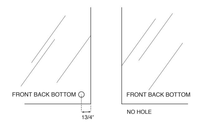
MEASURE THE GLASS SPACE BETWEEN EDGE OF GLASS AND CENTER OF HOLE. HOLE FURTHEST FROM EDGE GOES ON BOTTOM
