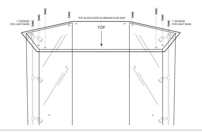
STEP 11. PLACE TOP GLASS DOOR ALUMINUM SLIDE GUIDE UNDER TOP GLASS.
