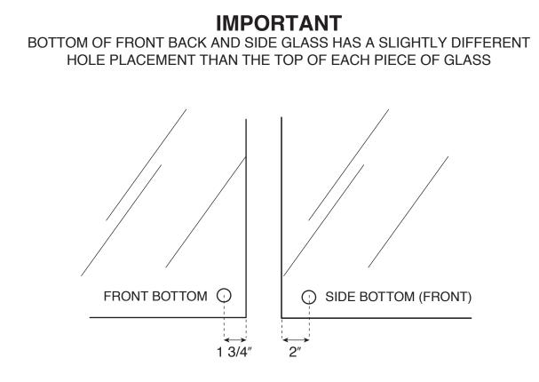
MEASURE THE GLASS SPACE BETWEEN EDGE OF GLASS AND CENTER OF HOLE. HOLE FURTHEST FROM EDGE GOES ON BOTTOM.
