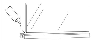
RUN BEAD OF ANY TYPE OF GLUE ON INSIDE (TOP) OF BOTTOM METAL SLEEVE. THEN TAP SLEEVES ON BOTTOM OF THE GLASS WITH A RUBBER MALLET.
