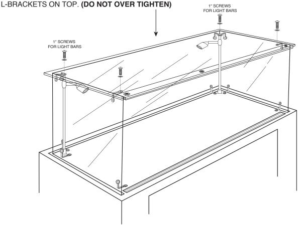
STEP 13. PLACE TOP GLASS DOOR ALUMINUM SLIDE GUIDE UNDER TOP GLASS.
