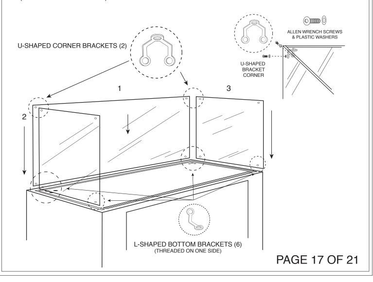
**STEP 11.** CAREFULLY SLIDE TOP GLASS ONTO PEDESTAL MAKING SURE YOU HAVE AN OVER-LAP ON BOTH SIDES.
