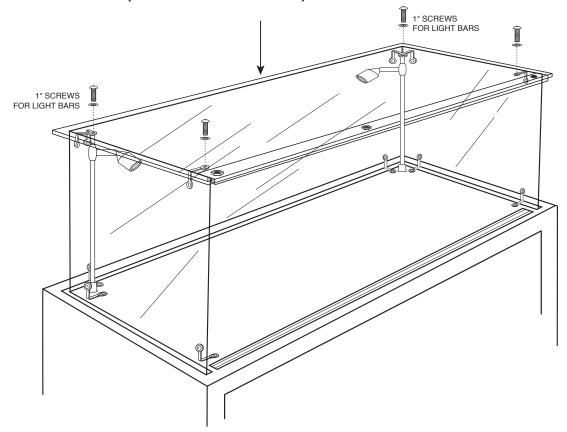
STEP 11. PLACE TOP GLASS DOOR ALUMINUM SLIDE GUIDE UNDER TOP GLASS.
