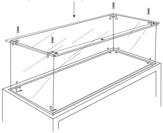
STEP 8. PLACE TOP GLASS DOOR ALUMINUM SLIDE GUIDE UNDER TOP GLASS.
