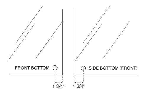
MEASURE THE GLASS SPACE BETWEEN EDGE OF GLASS AND CENTER OF HOLE. HOLE FURTHEST FROM EDGE GOES ON BOTTOM.
