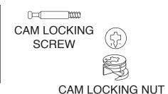
STEP 5. PLACE (4) CAM LOCKING SCREWS INTO (4) HOLES IN TIER 1-B BOARD.
