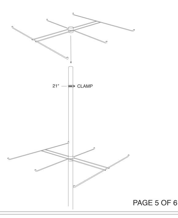
STEP 6. ATTACH THE WIRE SIGN HOLDER TO THE TOP OF THE RACK.
