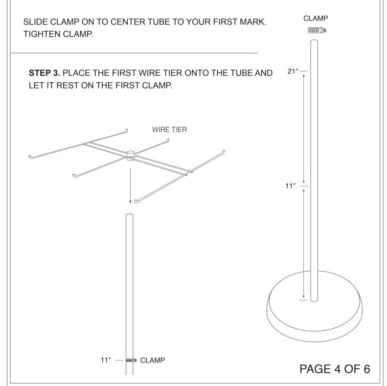
**STEP 4.** SLIDE THE SECOND CLAMP ON TO CENTER TUBE TO YOUR SECOND MARK AND TIGHTEN CLAMP.
